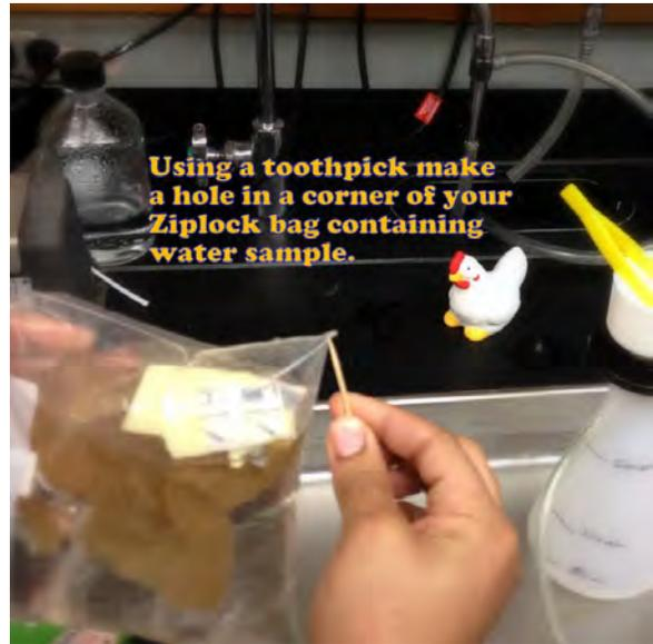
8. When everything is ready, turn the bag upside down and punch a small hole in the corner with a toothpick. Turn the bag over again and slowly add the water in a gentle stream directly to the middle of the filter, until it is completely wet it.
