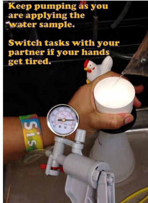
11. After about 300 ml of water have been filtered into the funnel, stop adding water. The picture at the right shows about how full the flask will be when it has 300 ml in it.
